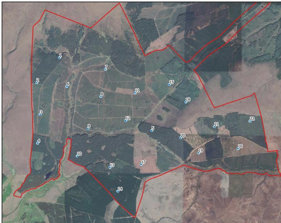
Figure 4. Third and Final Turbine Layout
